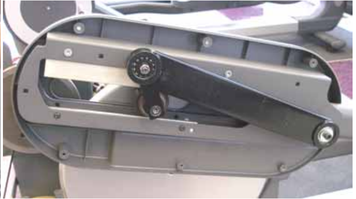
Fig. 9: attach the opposite end of the control link assembly Fig. 10: new control link assembly installed.
